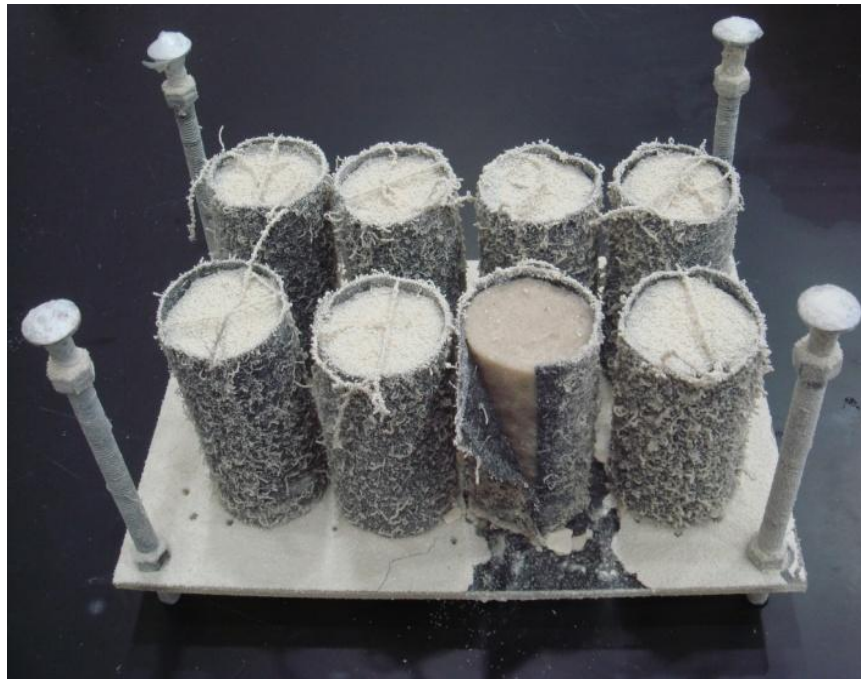
Figure 2-8 Photograph of specimens in the full contact flexible molds: (a) before the reactions; (b) after the MICP reactions. The full contact flexible mold was fabricated by geotextile. PVC shelf was used to support full contact flexible molds.
