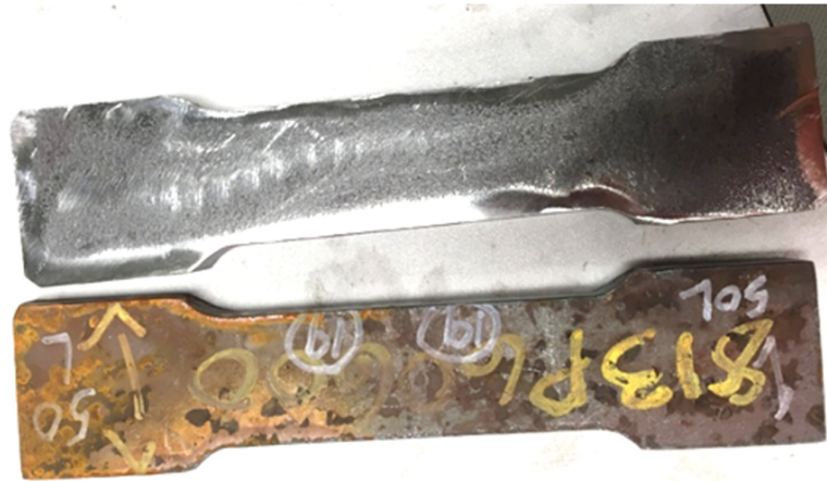
Figure 39. Corroded (bottom) and uncorroded (top) steel surfaces
