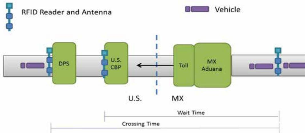
**FIGURE 14 Border crossing radio frequency identification system.**
