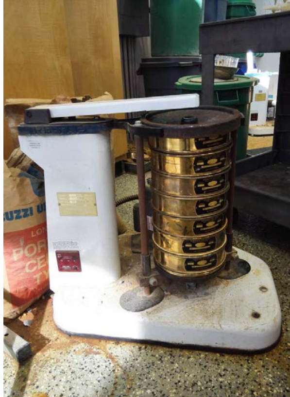
Figure 3.2 Sieve analysis at the Geotechnical Engineering Laboratory
