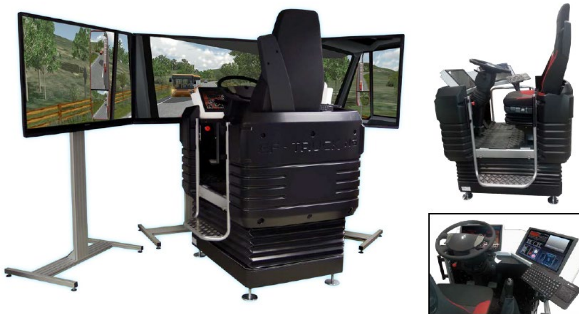
Figure 1. EF-Truck full motion driving simulator available at the City of Fayetteville Library 2
