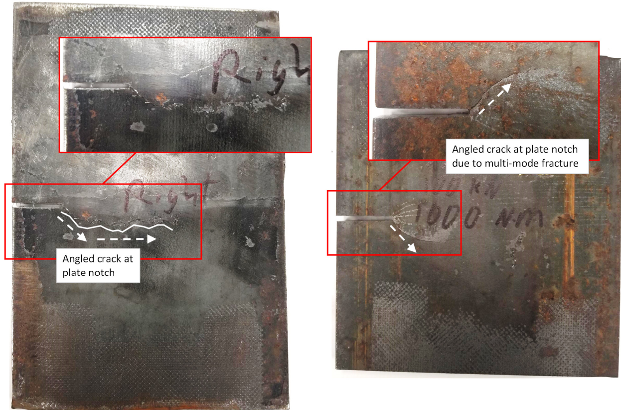
Figure 22. Resulting fatigue crack growth in un-retrofitted and retrofitted notched plate specimens under combined axial and torsional loading.
