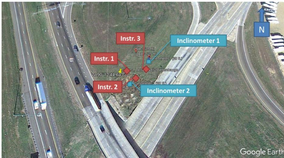
**Figure 4.15** Instrumentation layout at Slope 2 in 2018
