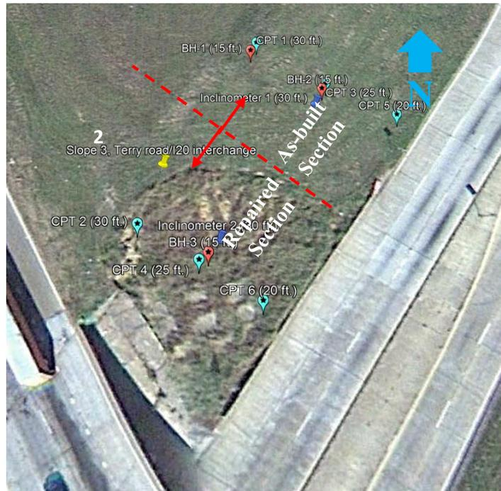
**Figure 4.10** CPT and borehole locations at Slope 2
