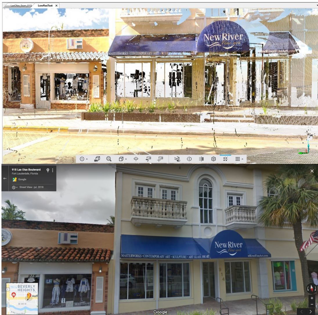
Figure 7: Comparison between what we see in the LIDAR scanned 3D view (top figure) and what Google Street View actually provides (bottom figure)
