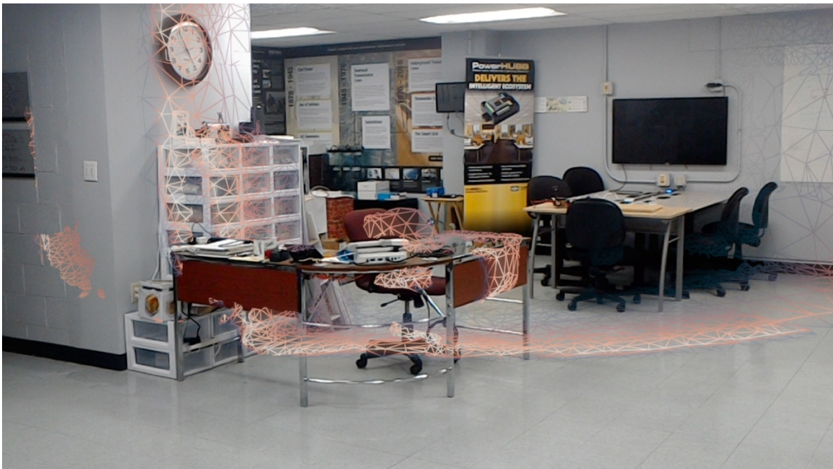
Figure 31: Microsoft HoloLens performing a mesh scanning of where we pointed our gaze
