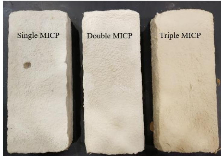
Figure 3-17. Surfaces of single, double, and triple MICP-treated samples after accelerated erosion.
