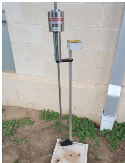
Figure 2-17. Photograph of dynamic cone penetrometer
