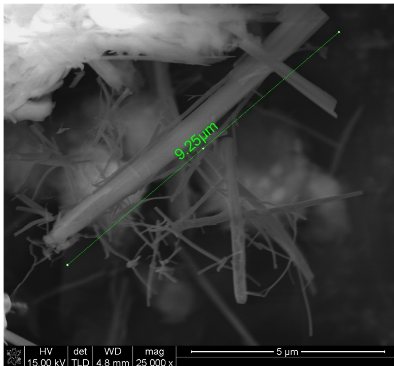
Figure 27: SEM image of ettringite crystals in BCSA soil-cement at 1-day
