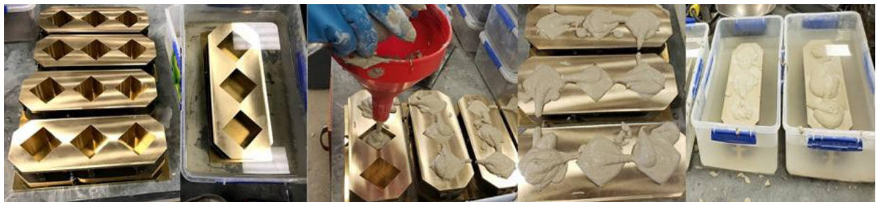
Figure 3: Fresh mortar specimen casting set-up.
