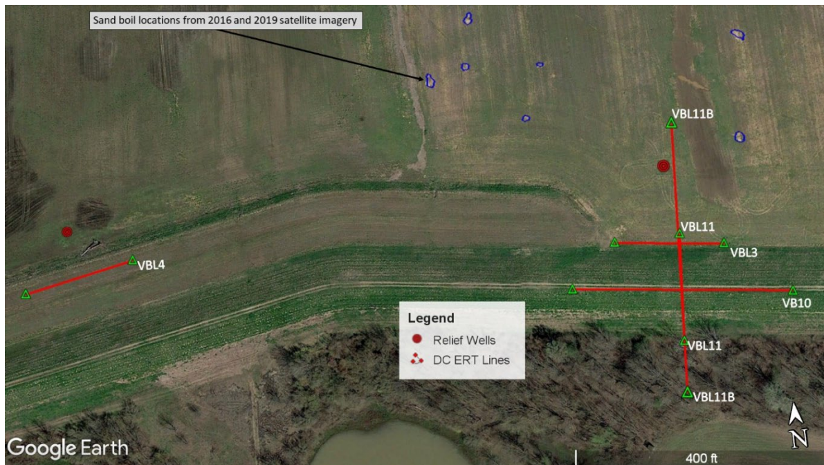
Figure 21 Control area DC ERT lines
