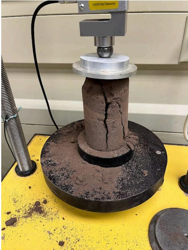
*Figure 2. Sample compacted after initial setting time*
