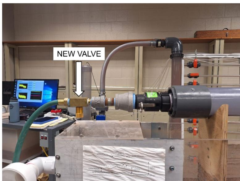
*Figure 7. Hose-valve-upstream chamber with connection for final setup*
