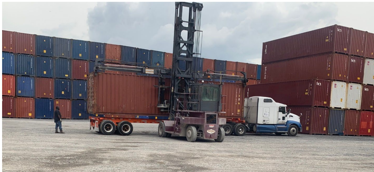
Figure 8: A side-loader mounts a 40' container onto a compatible intermodal chassis.
